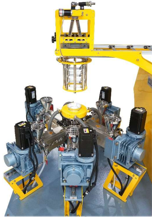
PICTURE ABOVE SHOWS OUR NEW ULTRA MICRO 5-LAYERS COEX FILM BLOWING LINE
